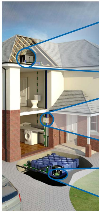
The Rain Director® saves energy and prolongs pump life as most rainwater harvesting systems stop and start the pump every time a toilet is flushed or water is demanded.
