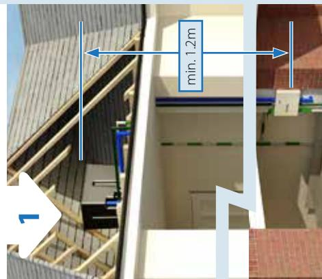
Locate the control panel where the rainwater enters the building on a wall in a frost protected area. (at least 1.2m below header tank)
