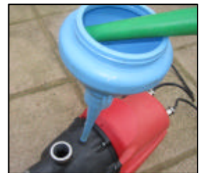
Fill the pump with clean water (needs about 5 litres) and replace the cap
