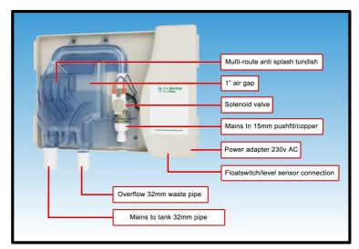
For this reason all mains backup devices must have an air gap where the mains water flows into the rainwater tank. The air gap in this system is an anti-splash tundish and overflow incorporated into one; the transparent blue moulded part. The level sensor is provided with 20 metres of cable and uses a push connection under the right hand panel.
