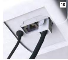
**10)** Connect the Cat 5 cable to connector **(H)** at the control panel and similar connector at the header tank.
