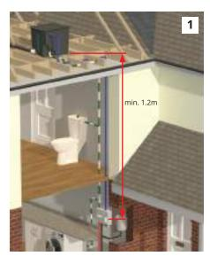
1) Locate the control panel where the rainwater enters the building on a wall in a frost protected area (at least 1.2m below header tank).
