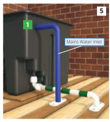
**5)** Connect the mains water outlet from the control panel **(E)** to the header tank mains water inlet **(1)** using 1/2 inch BSP.
